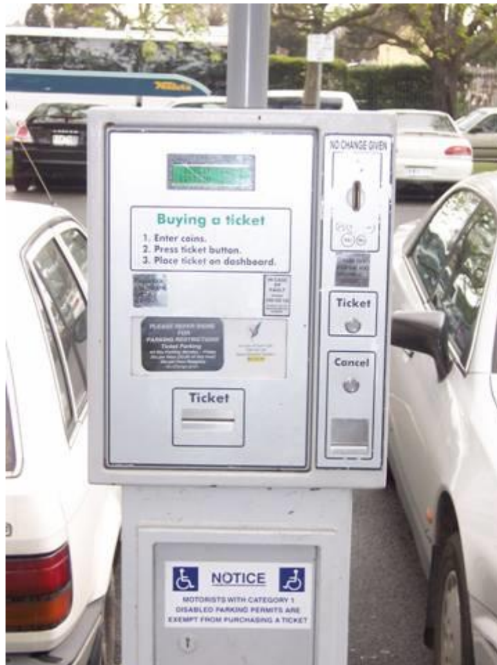
Figure 9: ‘The Ticket Machine’ prominently displays the algorithm or script the user must follow to be legally parked. As the user inserts coins the window above the sign displays how much time they have paid for.
